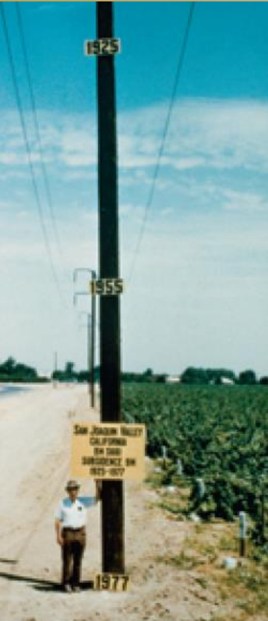
Figure 18 The marks on the utility pole indicate the level of the surrounding land in years past. Between 1925 and 1975 this part of the San Joaquin Valley sank almost 9 meters because of the withdrawal of groundwater and the resulting compaction of sediments.
