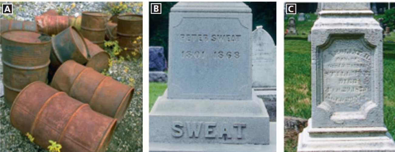
Figure 6 A Oxygen reacted with the iron in these barrels, forming iron oxide, or rust. B This granite gravestone, placed in 1868, shows little evidence of chemical weathering. C The inscription date (1872) on this marble gravestone is nearly illegible due to chemical weathering.
