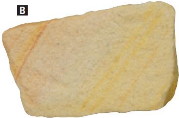
Figure 10 Although these two rocks appear quite different, both formed when sediments were dropped by moving water. A Conglomerate is made of rounded pebbles cemented together. B Sandstone is made of sand grains cemented together.
